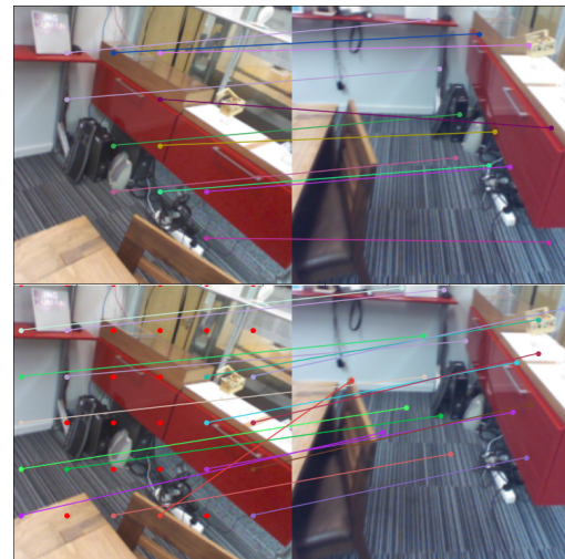
Figure 8. Predicted correspondences using 7-Scenes dataset [9]. This dataset was unseen by the network. On the top pair we can see the predicted matches and in the bottom the ground-truths. The red dots indicate that they are not visible. Due to sensor noise, some of the ground-truth visibilities are incorrect.
